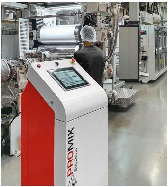
**Photo caption**Promix Microcell Technology on an extrusion line for packaging films.
