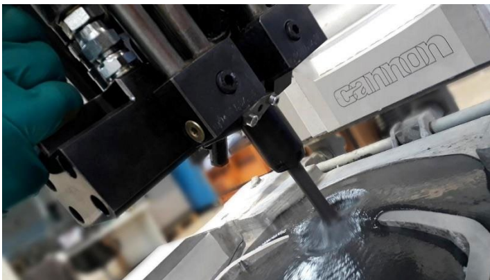
Cannon Afros has extended the range of its EG-AX multi-component mixing head system for expandable graphite to include viscoelastic foams, continuous sandwich panels and poly-iso boards. Photo Cannon Group
